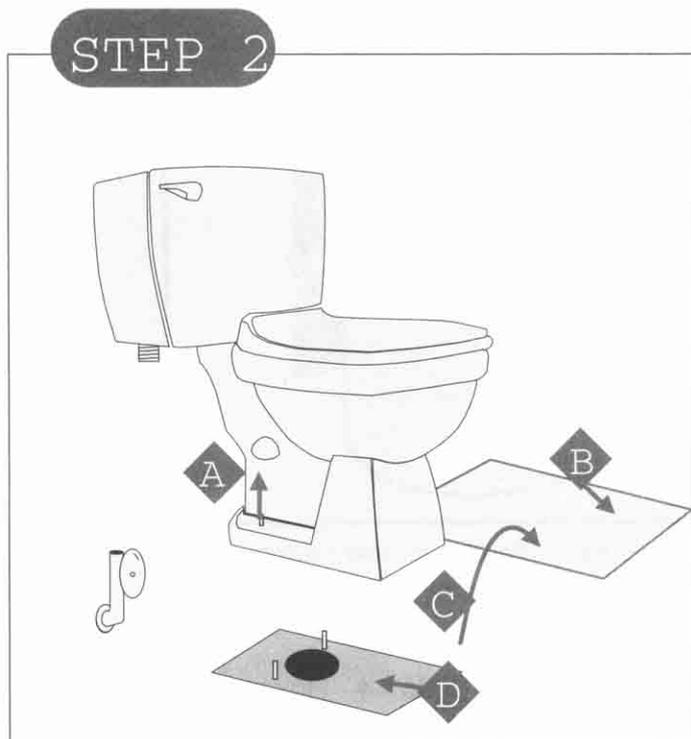
**STEP 2:** Disassemble Toilet from Floor
